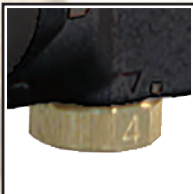
Air Regulator 4 torque setting.
