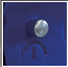
SAS (Side And Side) System Forward / Reverse for one hand operation.
