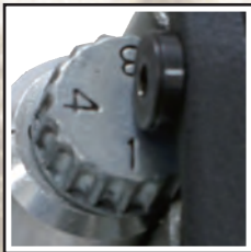
Air Regulator 4 torque settings.
